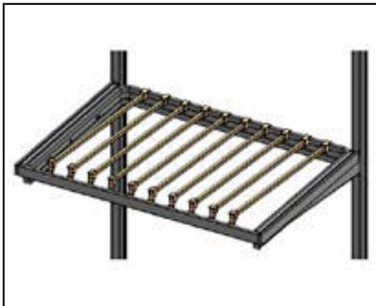
Position all Rods into the Gliding Frame. Rods can be adjusted by sliding sideways.
