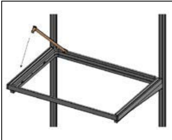
Position Rod, clipping the back hook over the back part of the Glider.
