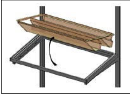
Drop Shoe Rack in place, starting with the back side.
