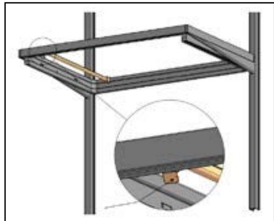
Push the locking tab up to remove a Rod.
