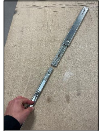
Push down on the black plastic part and remove the inner Drawer Slide.
